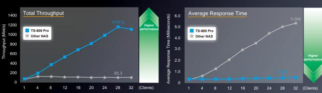
The NetBench test result shows the TS-809 Pro delivered a throughput of 1177.3 Mbit/s and an average response time of 0.397 milliseconds when 28 clients were accessing the NAS simultaneously.
