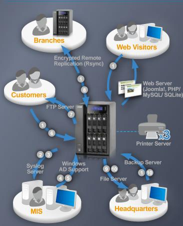
The TS-809 Pro supports file sharing across Linux, UNIX, Mac, and Windows platforms. Versatile business functions are supported, e.g. file server, FTP server, backup server, printer server, web server, encrypted remote replication by Rsync and Windows AD (Active Directory). SSH login and web page SSL login enable users to transfer, store, and share data securely. The NAS supports UPS devices to prevent avoid critical data loss when power outage occurs during data transfer.
